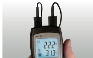
Simultaneous recording of temperature by two connected probes and display of differential temperature
