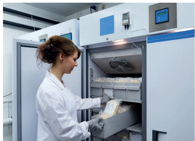
With its large measuring range of up to -100 °C, the 176 T2 is also able to accurately monitor the storage of blood plasma.
