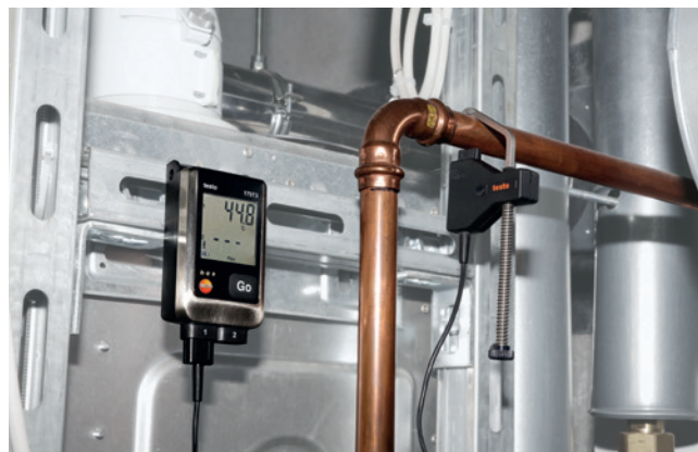
The temperature data logger testo 175 T3 with a clamp probe fitted to a shower water pipe.
