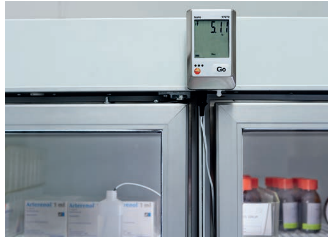
The probe is placed in a glycol solution to simulate the storage temperature of liquid products.
