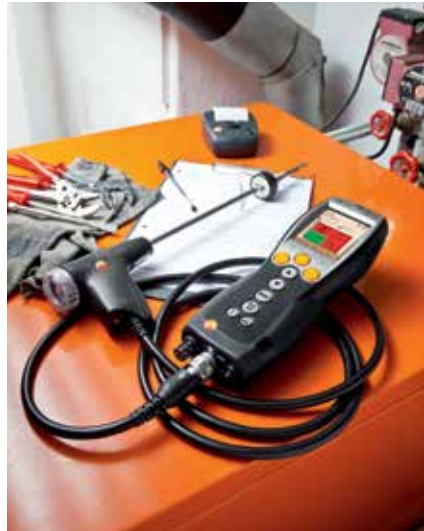
Fig. 19: All key readings and calculation values can be calculated simply and precisely using a flue gas analyzer.
