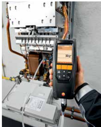
Fig. 15: As well as flue gas readings, the testo 320 flue gas analyzer can also be used to measure absolute and differential pressures quickly and precisely.
