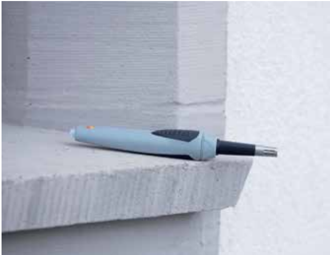
The outside temperature is transmitted to the testo 635 by a wireless probe.
