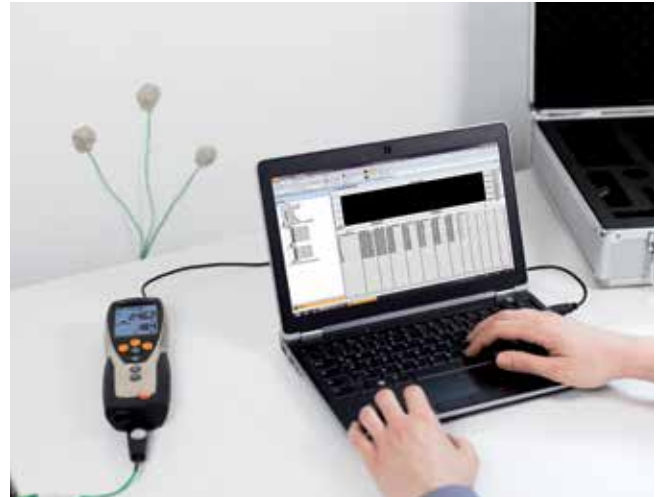
The development of the U-value can be followed in real time with the testo ComSoft software.
