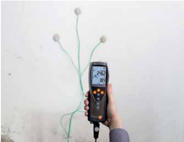
The different temperatures come together in the measuring instrument testo 635, and the U-value is calculated.
