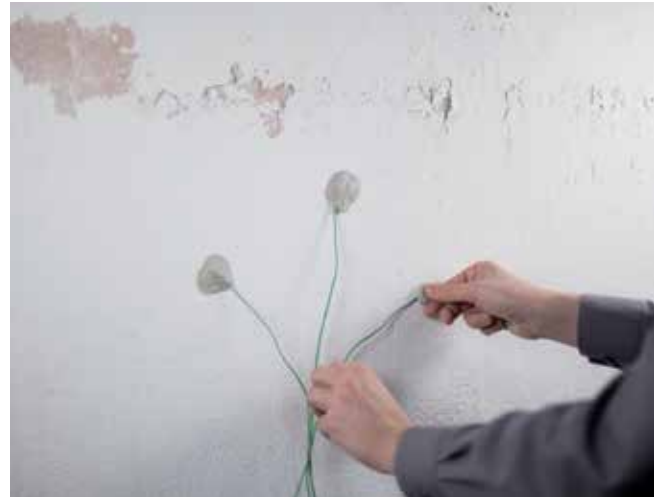
The U-value probe determines not only the temperature of the wall, but also the indoor room temperature.
