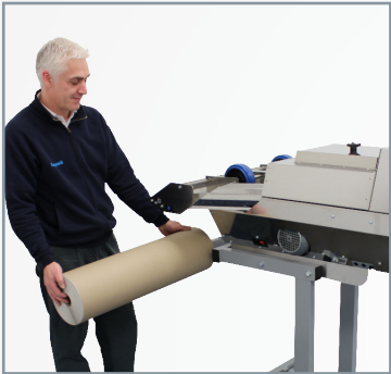
Place the roll of paper on the holder
