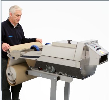
Feed the paper through the rollers
