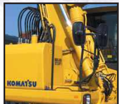
Large handrail for safe access
