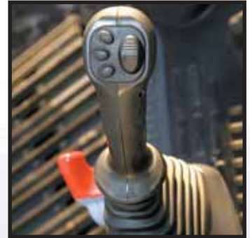
Joysticks with proportional control button for attachments
