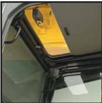
Large sun roof with integrated sun shade
