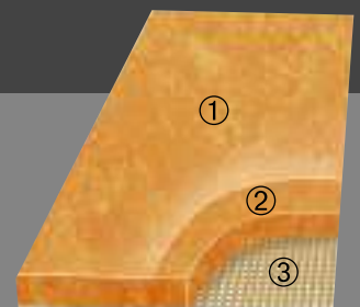
Linoleum xf construction
