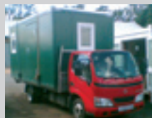
2. ASSEMBLED UNIT CAN BE TRANSPORTED BY TRUCK OR FORKLIFT, OR LIFTED FROM ITS LIFTING EYES BY CRANE
