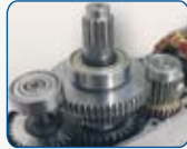
Thermo treated gears on rotating arms supported by ball bearings;
