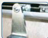
Adjustable, mechanical limit switch in opening and closing
