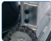
Mechanical limit switch with chain transmission of easy adjustment
